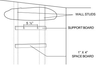
Fig. 1 - Mounting the Heater
